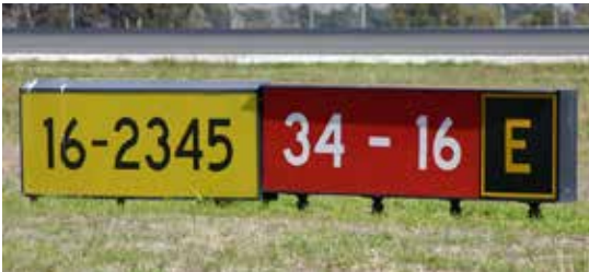
Movement Area Guidance Sign (MAGS): you are at the Holding Point for Runway 34-16 on Taxiway E with 2345m take-off run available on Runway 16.
